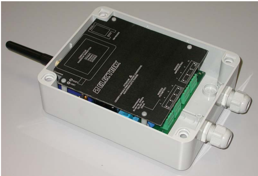
View of the inner protection panel
